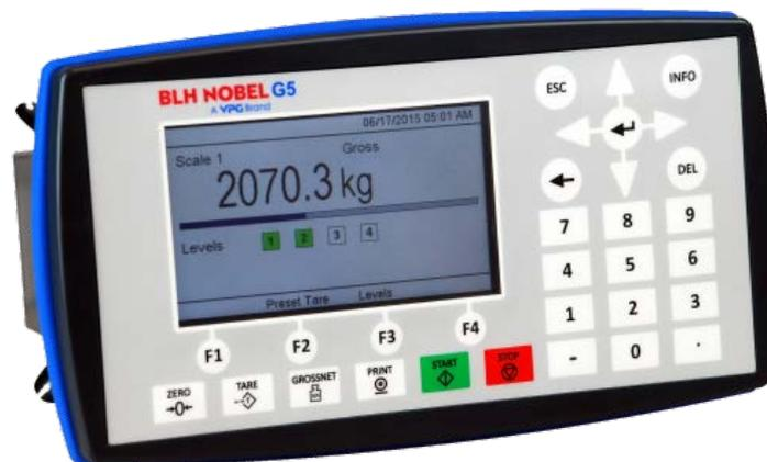
*Front panel of the G5 instrument with color display, four function keys below the display, six application specific keys, numerical keypad, joystick keypad (arrow keys), Esc, Backspace, Delete, Tab and ENTER keys.*
